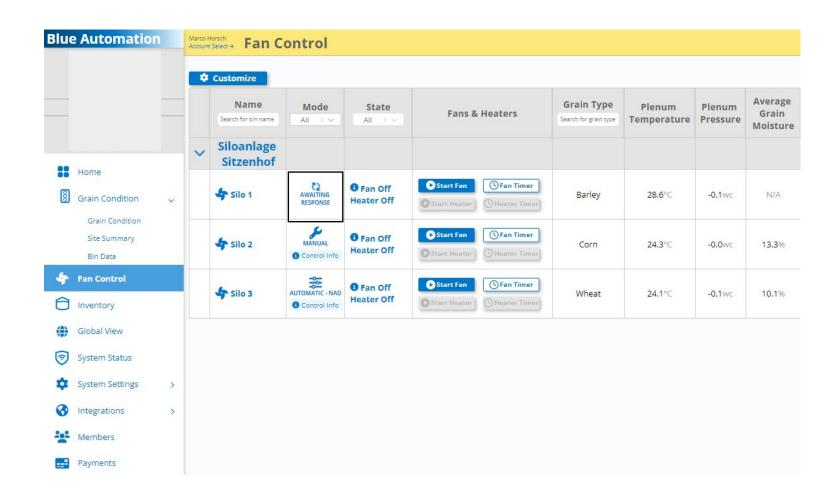
Step 8: The term "Awaiting Response" now appears in silo 1 under the "Mode" split, which indicates that the system is now processing your settings. Please refresh the page again after a minute. The split should now have the Automatic-Aeration mode applied
